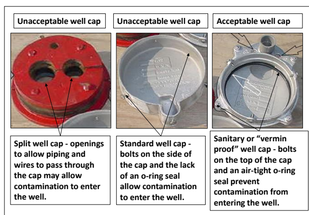
Figure 2: Photos of acceptable and unacceptable well caps
